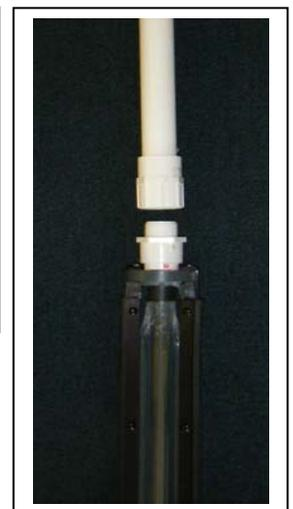
3. Bond the riser pipe to the disinfection chamber & allow the glue to set (upto 30 minutes). Usually, after a few minutes, the glue is sufficiently dry to allow light, careful, handling.
