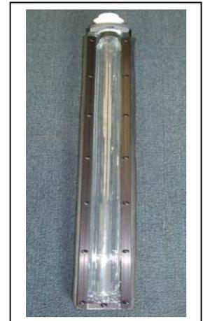
6. Slide the disinfection subassembly through the riser pipe into the disinfection chamber using the white PVC handle. Make sure that the subassembly is at right angles to the inlet and outlet pipes, and that the holes on the upper hub of the subassembly lock onto the two pins in the disinfection chamber. The orientation of the frame is very important for successful UV unit operation.
