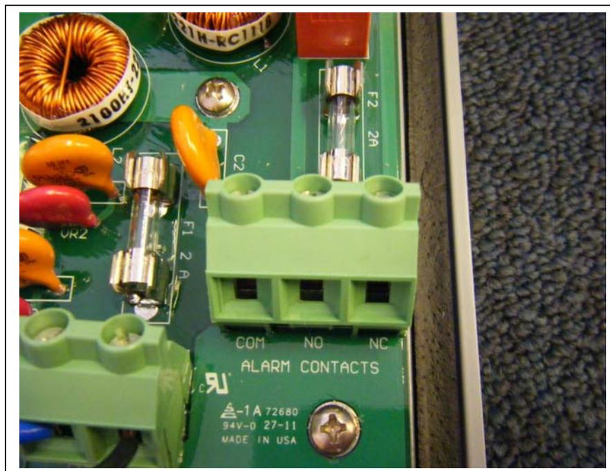
Connect alarm wires as needed for your specific circuit or application.
